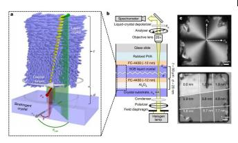
Apparatus measuring the Casimir torque. Credit: *Nature* (2018). DOI: 10.1038/s41586-018-0777-8
