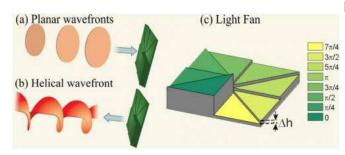
(a) The normal incident laser pulse has a planar (nontwisted) wave front. (b) After reflecting off of a spiral foil, the light has a helical (twisted) wave front. (c) The foil used in the simulation has eight parts to mimic a spiral phase plate. Credit: Shi, et al. ©2014 American Physical Society
