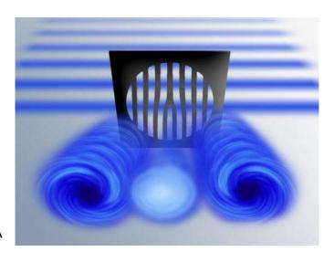
In the past, special grid-like masks were used to create vortex-beams.
