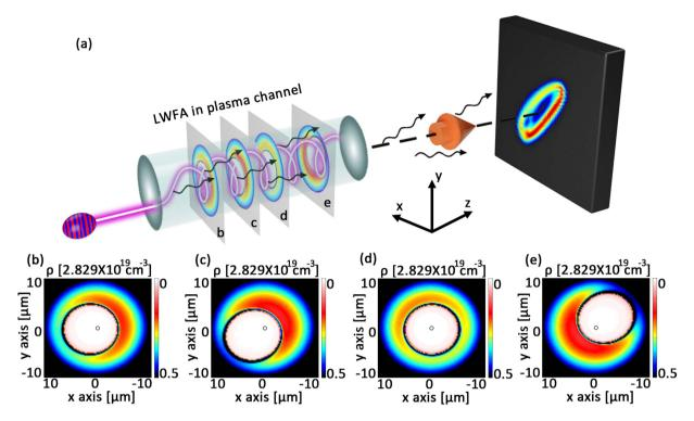
Figure 1. Sketch of the radiation source from a helical plasma undulator based on LWFA. (a) Spiral motion of laser pulse, wakefield in the plasma channel and the far field X-ray radiation distribution. (b–e) are the electron density distributions of the transverse slices of the accelerating bubble structure with largest radius at t = 133 fs (b), t = 600 fs (c), t = 1200 fs (d), t = 1800 fs (e).
