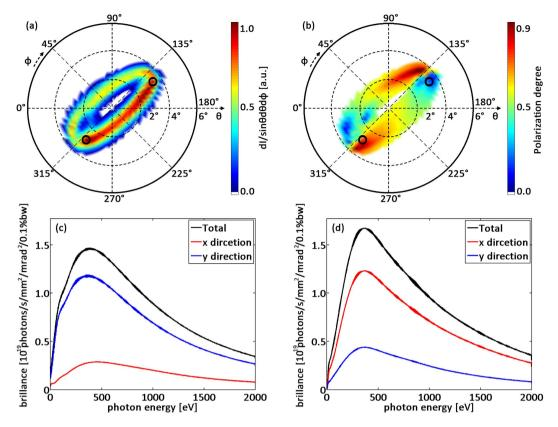
**Figure 3.** Intensity and polarization distributions of X-ray radiation. (a) Far field radiation intensity distribution, (b) polarization distribution, (c) radiation spectrum of the marked upper right point and lower left point (d).
